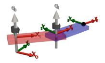
A robot can be described as a sequence of links which are attached to joints.
