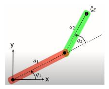
Velocity of End-Effector in a 2-Joint Robot Arm (2D) - cont'd
