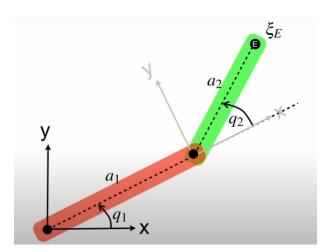
Given the position of the end-effector  $(x_E, y_E)$  you are asked to calculate (using Python and the robotics toolbox we have been using) the required joint angles to achieve this position.
