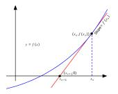
Then the approximated solution for finding the root of f (where f(x) = 0) can be calculated iteratively by:
