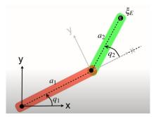
Given the position of the end-effector  $(x_E, y_E)$  calculate the required joint angles to achieve this position.
